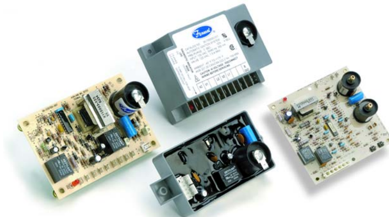
FIGURE 4: Typical DSI controls for 12 VDC, 24 VAC and 120 VAC. Note the large cylindrical spark transformer that generates the high voltage ignition spark.
